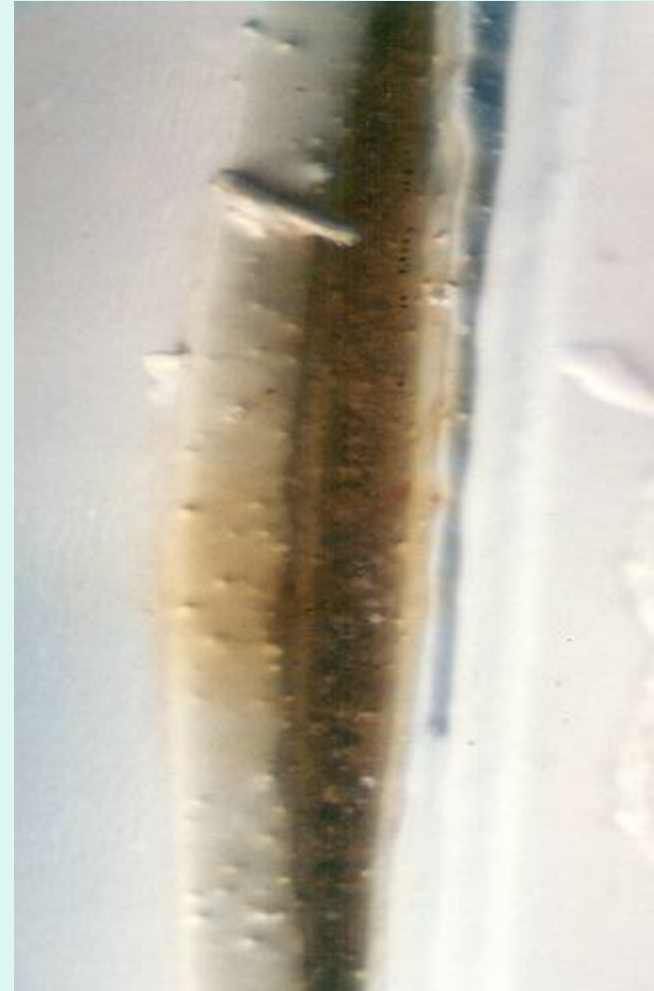
1 yr old 3 coat zinc epoxy urethane over pack rust
